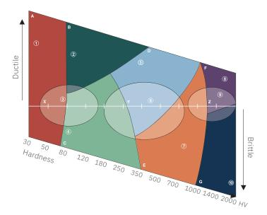
Find the hardness of your material on the X-axis, then move up or down the Y-axis, depending on its ductility. Learn more and see optimized methods for your material at <u>Struers.com</u>
