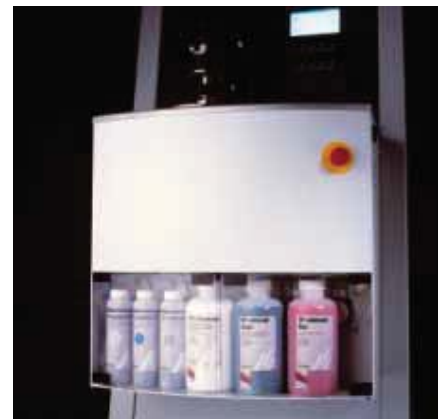
AbraPol-10 includes an integrated dosing unit for Diamond Suspension and Lubricants
