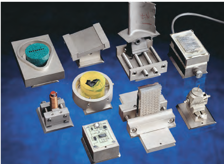
A wide range of specimen holders can be used on Accutom machines
