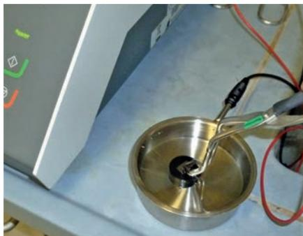
**Fig. 6:** Electrolytic etching of the mounted samples using the "tip" procedure (non-conductive mounting resin works as insulator to cathode, which is the bowl = container).
