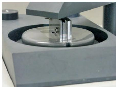
**Fig. 4:** Sheet metal bundle on electrolytic polishing device.
