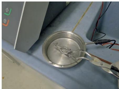
**Fig. 7:** Electrolytic etching of sheet metal bundle without mounting of the samples using the "dip" procedure.
